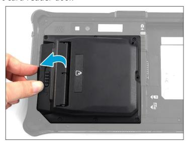
13. Slide the smart card reader lock switch to the lock position.
