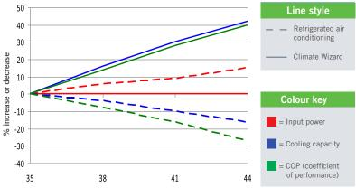
Outdoor Temperature (Degrees Celsius DB) Source: Uni SA Roxby Downs Report June 2009 Climate Wizard's cooling performance can rival that of refrigerated systems, using up to 80% less energy.
