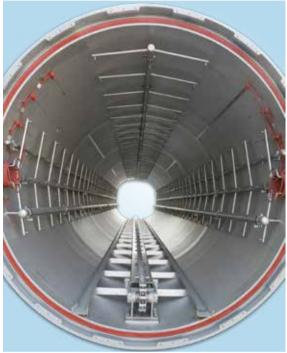
Side Sprays for Fish Cooling & Spray Manifolds for Vessel Cooling
