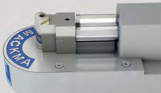
Simple mechanical locking screw for bend stop position
