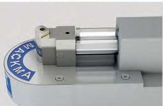
Simple mechanical locking screw for bend stop position
