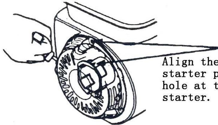
Align the arrow on the starter pulley with the hole at the top of recoil starter.
