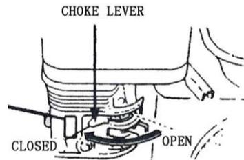
To restart a warm engine, leave the choke lever in the OPEN position.
