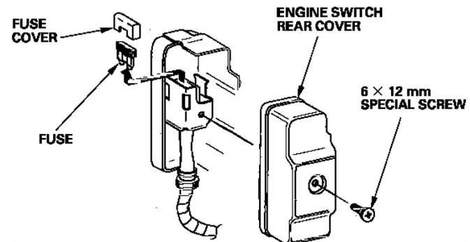
Frequent fuse failure usually indicates a short circuit or an overload in the electrical system. If the fuse burns out frequently, take the engine to a servicing dealer for repair.
