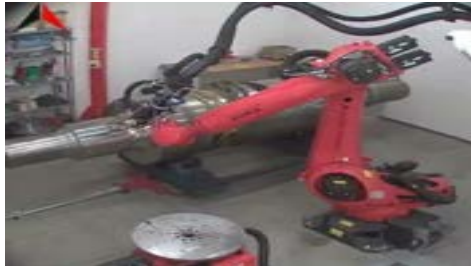
LASER POWDER DEPOSITION WELDING ON A ROLLER
