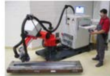
MOBILE LASER HARDENING ON A BENDING TOOL
