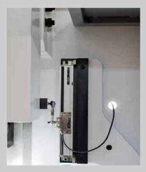
**5** Patented throat distortion compensation device
