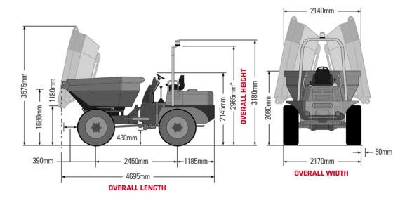
MAX SAFE CARRYING WEIGHT: 6000KG | LEVELLED CAPACITY: 2360L | HEAPED CAPACITY: 3130L
