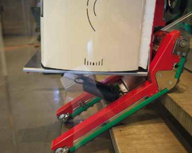
DOMINO is equipped with non-scratching, anti-slip crawler tracks that can rotate 360 degrees. Made of highly resistant special compound, allows you going up and down any type and shape of stairs with ease and safety.
