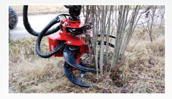
The EG250 heads are an efficient combination of a felling head for energy- and small wood and a traditional loading grapple. The head is suitable for all kinds of clearing and thinning operations as well as felling, collecting, handling and loading of trees and bushes etc. Thanks to the normal claws and the knife, even larger bushes and branches can be taken down with one cut. Very easy to install because of no need for any additional hydraulics.
