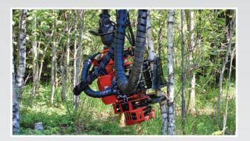
This is a giant leap forward in professional energy- and small wood harvesting. With this unique head you cut small bushes, twigs and thinner trees with a snap and fell bigger trees using the saw. The head also works perfectly as a traditional loading grapple. The XG220 is a combination of two of the most successful and tried out Mecanil products; Mecanil EG250 energy wood felling head and SG220 grapple saw.
