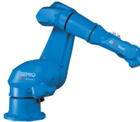
The range of 6-axis polyarticulated robots: 6X Visual combined with the Sepro Visual 3 control platform offers a Premium solution for carrying out all tasks, from simple unloading to more complex applications. Sepro Stäubli polyarticulated robots are quick and precise. They are designed with a closed and naturally clean structure (ISO 5 as standard) for equipping 20-tonne to 1300-tonne injection molding machines.
