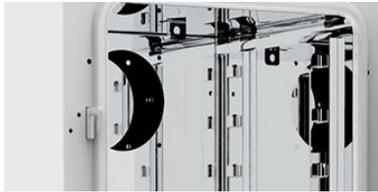
Interior is made of high-quality brushed stainless steel. Anti-slip diaphragm design & spacing adjustment, to avoid samples falling off when pulling the diaphragm.
