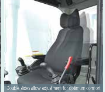
Double slides allow adjustment for optimum comfort
