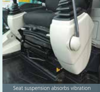
Seat suspension absorbs vibration
