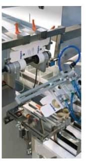
The **C222** is a side-load, intermittent motion cartoning machine suitable for manual or automatic packaging of pharmaceutical, nutraceutical, cosmetic and food products into pre-glued cartons.
