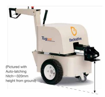
A powerful machine, the Tug Axis is available in one or two tonne towing capacities.
