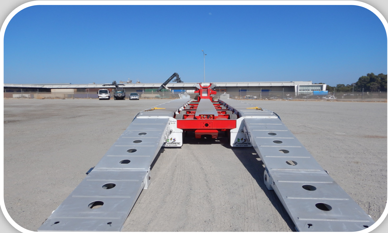
QUAD DECK WIDENER LOW LOADER 4 ROWS OF 4
