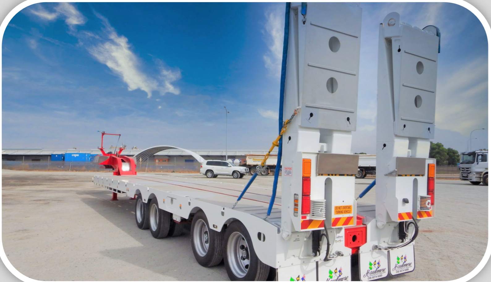
QUAD DECK WIDENER LOW LOADER 4 ROWS OF 4
