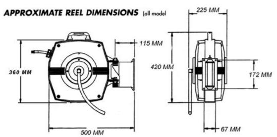
Length 580mm, Width 250mm, Height 500mm, Mass 10kg
