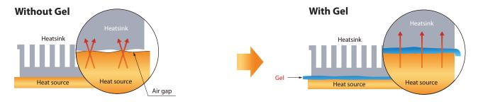
Hard thermal conductive sheet stresses IC and PCB.
