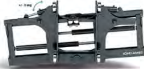
Carriage with center leveling (2 forks) for sensitive cargo
