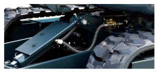
Two-Piece Hose for the Dozer Cylinder Two piece hoses were applied for a better and easier maintenance.
