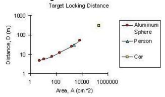
Maximum target distance is determined by the size and shape of the target. The sensor can see an average size car at about 300 meters (1,000 feet).
