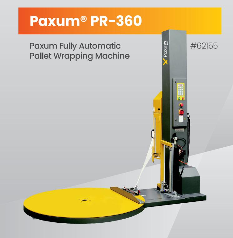
8 Wrapping Programs 250% Power Pre-Stretch Remote Control Operation Digital Touch Control Panel
