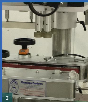
Servo driven Bottle clamp belt mechanism- 2"
