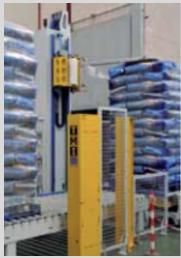
The Ilergir automatic pallet wrapper is a turntable wrapper designed for pallets of bags, which integrates into the bagging line. It has an automatic sealer to fasten the end of the wrap, it can be supplied with an optional top cover applicator for a weather proof seal, also a corrugated cardboard wrap for extra protection.
