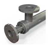
The HRS DTR Series is a complete stainless steel double tube heat exchanger designed for industrial and environmental applications. The product flows through the inner tubes and the service fluid flows through the surrounding shell. As a result of its geometry, the DTR Series has a continuous free-pass cross section allowing large particles to be processed and reduces the risk of product blockages.
