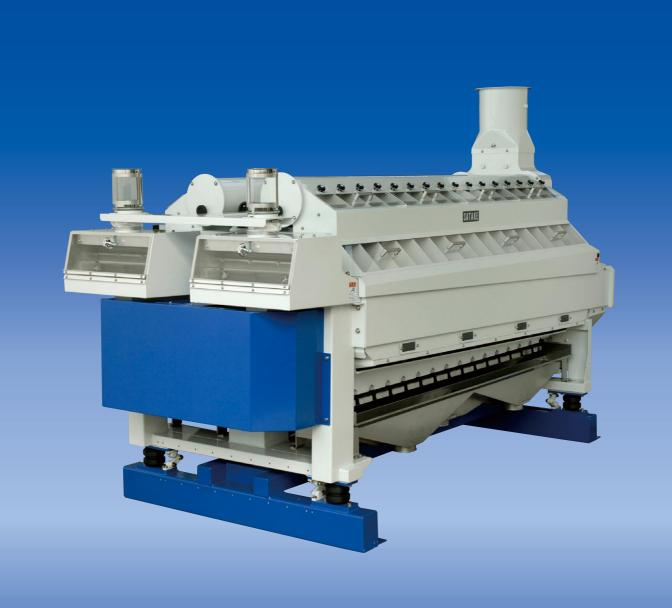
The Satake SPU Purifier is a newly redesigned state-of-the-art purifier which uses vibratory action to efficiently remove bran from middlings and semolina. It represents another step forward in the evolution of Satake's flour milling technology, and boasts a number of significant improvements over previous models.
