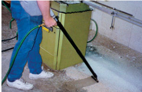
Model 6192 Vac-u-Gun Collection System with bag vacuums absorbent and chips.
