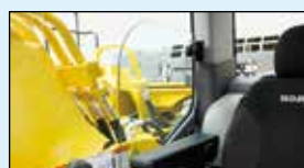
One-touch storable front window lower glass
