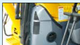
Defroster (conforms to the ISO standard)
