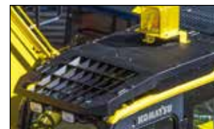
Bolt-on Top Guard OPG level 2 (ISO 10262) for falling object protection.
