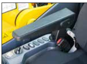
Remote intermittent wiper with windshield washer
