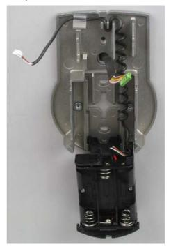
7. Position the cover on top of the base plate in an angle >90°.
