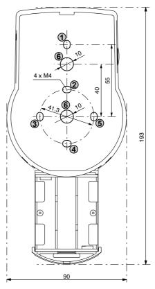
Drill the 3 fixation bores Ø3.2 x 14 mm and the cable leadthrough bore Ø10 mm. Remove burrs. Tap M4 threads into the 3 fixation bores. Remove the 3 screws on the bottom of the cover (1 at the battery compartment, 2 at the housing). Lift-off the cover from the base plate, then carefully remove the battery compartment.
