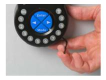
12. Check battery compartment for proper movability: carefully push the battery compartment into place, then slide it out again Do not insert the batteries and do not fix the battery compartment screw yet.
