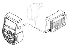
In its standard version the electronic safe lock Axessor USB is battery powered and consist of: the **input unit**, the **lock** and the **connection cable**. The lock includes 2 inputs and 2 outputs (assignment → External connections at the lock on page 23). Optionally, an external power supply (6VDC/500mA) can be connected to one of the lock sockets "X1" or "X2".
