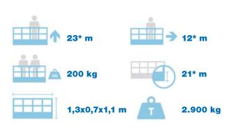
$<sup>^{\</sup>star}$  outreach and height max values and repeatability can change within  $\pm\,3\%$  due to manufacturing variation and working condition.
