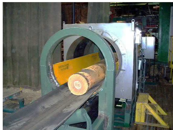
Round shape for optimal detection of metals in tree trunks.
