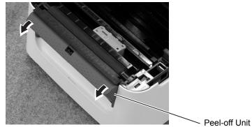
**3.** Remove enough labels from the leading edge of the media to leave 20 cm of backing paper free, and insert the top edge of the backing paper into the media slot in the Peel-off Unit as shown below.
