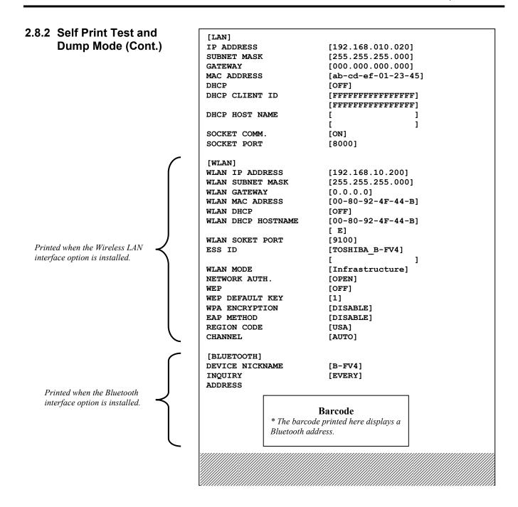
The test print content are different based on the emulation mode. The list below is for TPCL mode.
