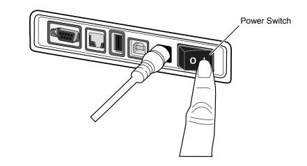
**2.** As the printer powers on LED 1 and 2 will lite first in orange then off and finally LED 1 should stay illuminated in green.
