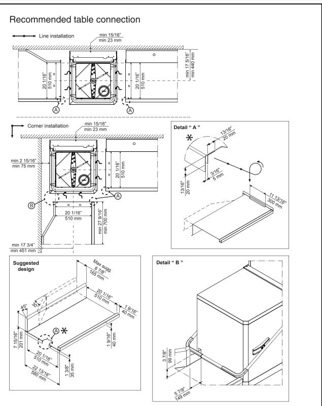
All tables must be connected to the dishwashing units according to local regulations and industry standards which may differ from the recommendations herein suggested. Electrolux Professional is not liable for any failure in complying with local design standards. Doc Nr : 59566BF00
