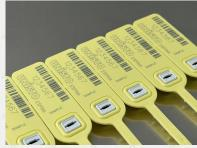
A pull-tight variable length security seal with unconventional fish-bone ribbon design to maximize tamper evidence and unparelled security feature with its unique 4-prong metal jaw which cuts through ribbon upon pull-back attempt. Revolutionary locking jaw ensure no reverse sealing secured by heat welding. Calibration in centimeter on the ribbon strap makes cutting and welding on the ribbon visible.
