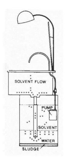
The unique parts washer filtering system uses the principle that a petroleum-based solvent is both insoluble in and lighter than water. While the unit is in operation, the solvent is continuously recycled as shown in the above sketch. As the used solvent returns to the water, via the drain tube, droplets are formed that rise back up to the main body of solvent. The water retains the particles and impurities that then fall to the bottom.
