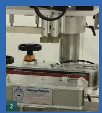
Servo driven Bottle clamp belt mechanism-2"
