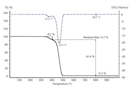
TGA measurement on BR at a heating rate of 10 K/min in nitrogen (40 ml/min), from 800°C to 1000°C, the measurement was continued in synthetic air; sample mass amounted to 9.90 mg; crucible made of alumina.
