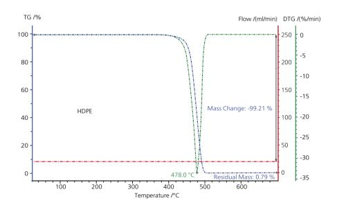
Decomposition behavior of polyethylene in a nitrogen atmosphere, illustrated by the TGA, DTGA and gas flow curves; heating rate 10 K/min
