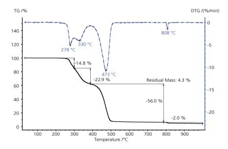
TGA measurement on CM at a heating rate of 10 K/min in nitrogen (40ml/min); from 800°C to 1000°C, the measurement was continued in synthetic air; sample mass amounted to 9.94 mg; crucible made of alumina.
