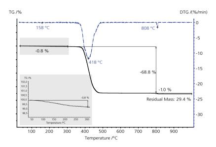
Picture-in-picture plot of the measurement on PA66/GF, heating rate of 20 K/min in a nitrogen atmosphere (40ml/min), from 800°C to 1000°C the measurement was continued in synthetic air; sample mass 10.47 mg, crucible made of alumina.
