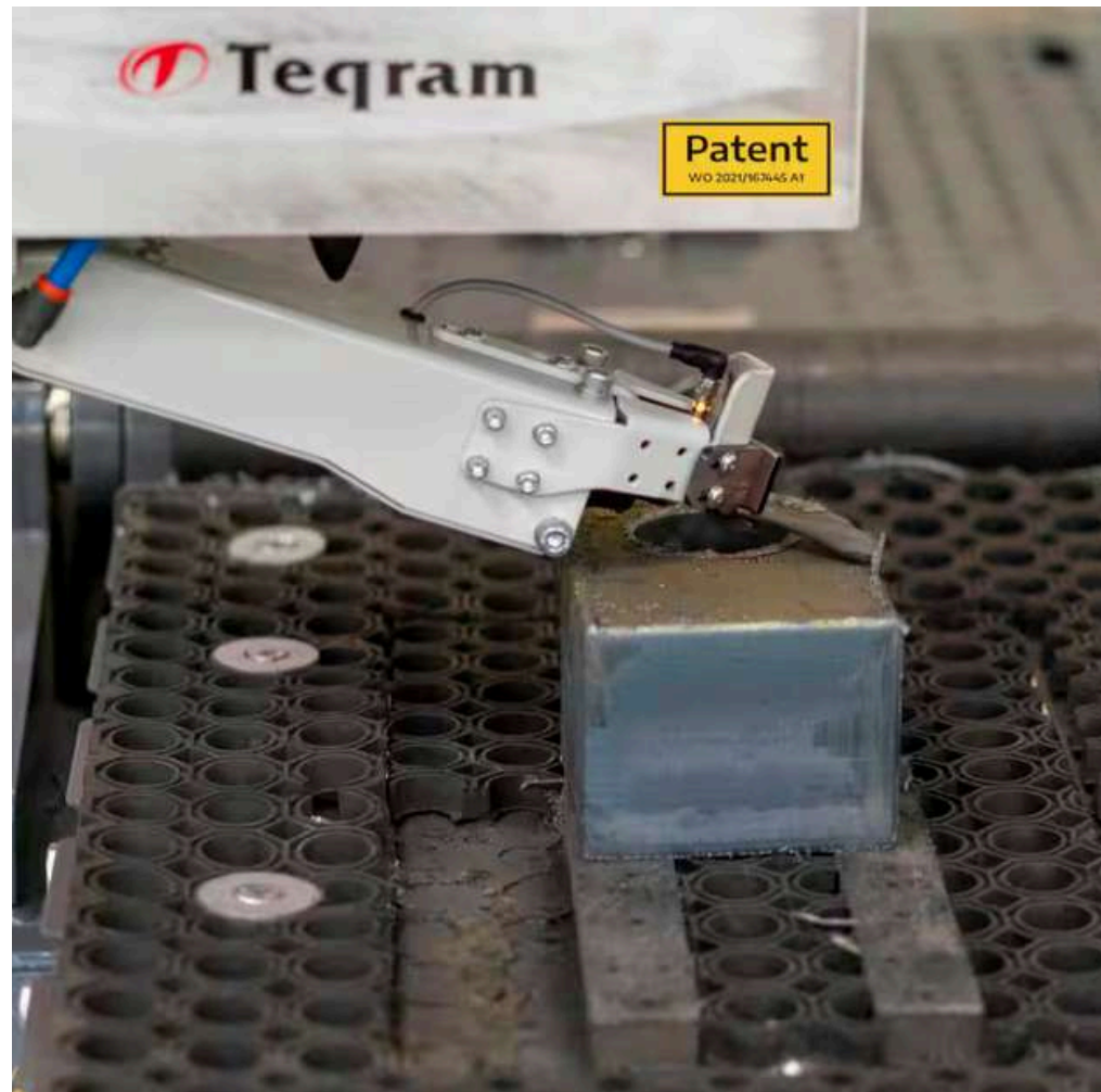
Robotic deslagging with chisel tool
