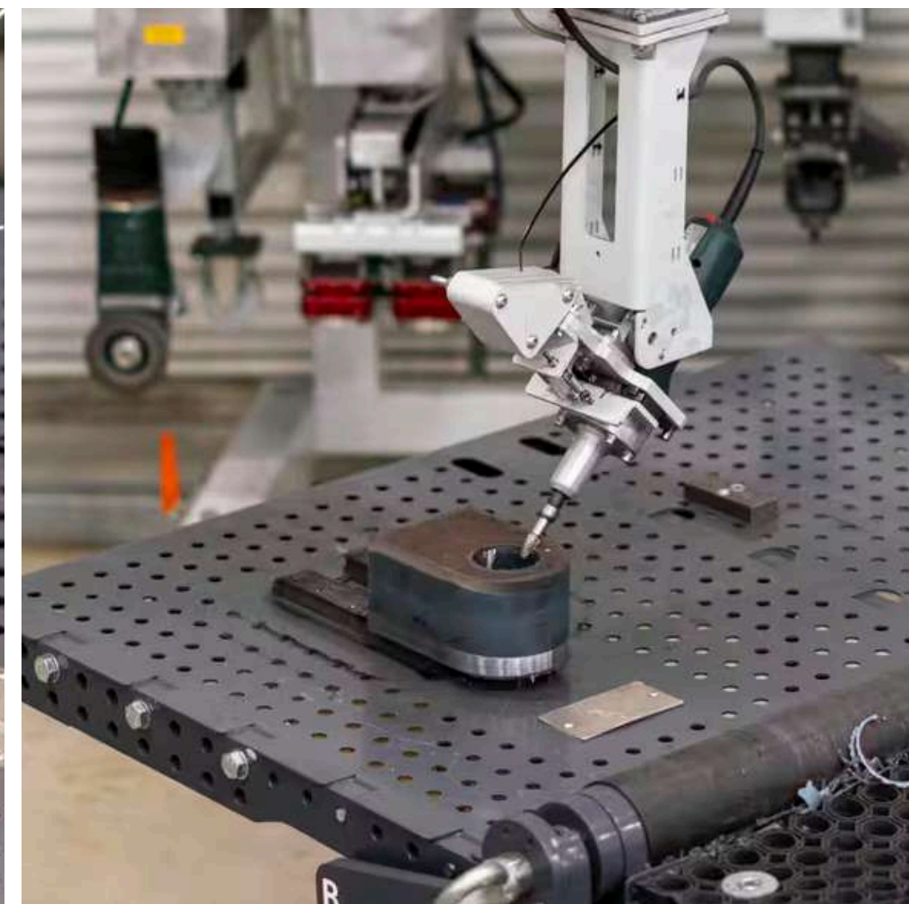
Edge-breaking, edge-rounding and chamfering with die-grinder
