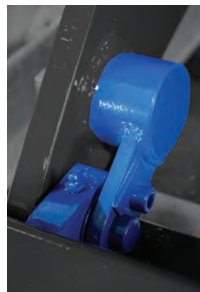
Bolt on hinge blocks upper and lower.
