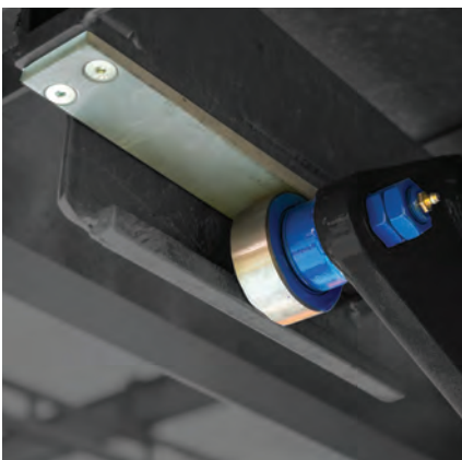
Greaseable Roller followers and Bisalloy 80 roller paths upper & lower.
