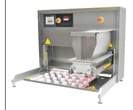
Mono Equipment's innovative Epsilon Tabletop Confectionery Depositor is one of the smallest tabletop confectionery depositor available — requiring just 950mm width of space in which to operate.
