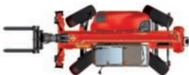
4 wheel drive for short turns in restricted areas
