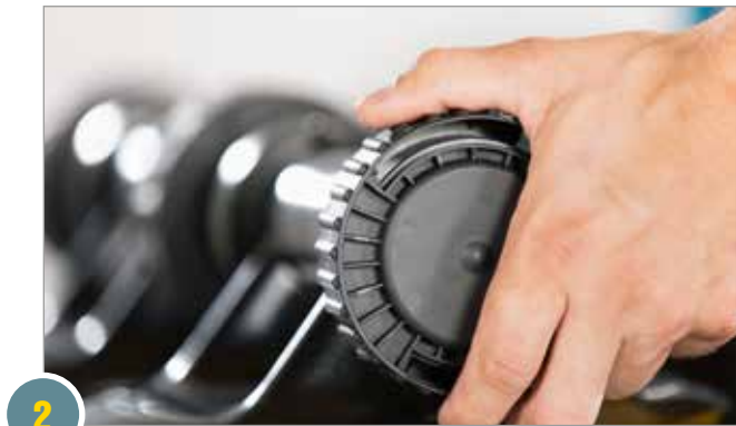
The clamping nuts on the cartridge screw connection are then loosened.
