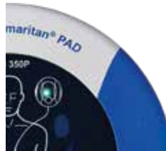
Figure 10. Flashing green LED; no action required.
