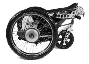
The Trekinetic GTE was designed to fold down and fit into a regular car. The front wheels come off with the simple click of a button and the rear castor folds down behind the seat. It has also been designed to fit into most larger vehicles with the wheels still on.
