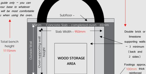
NOTE The aim is to have the benchtop level with the oven floor. Therefore the outside wall should be total bench height less thickness of whatever you are using to finish your benchtop eg. tile thickness.
