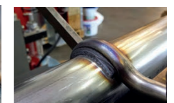
HD-MAG welding process
