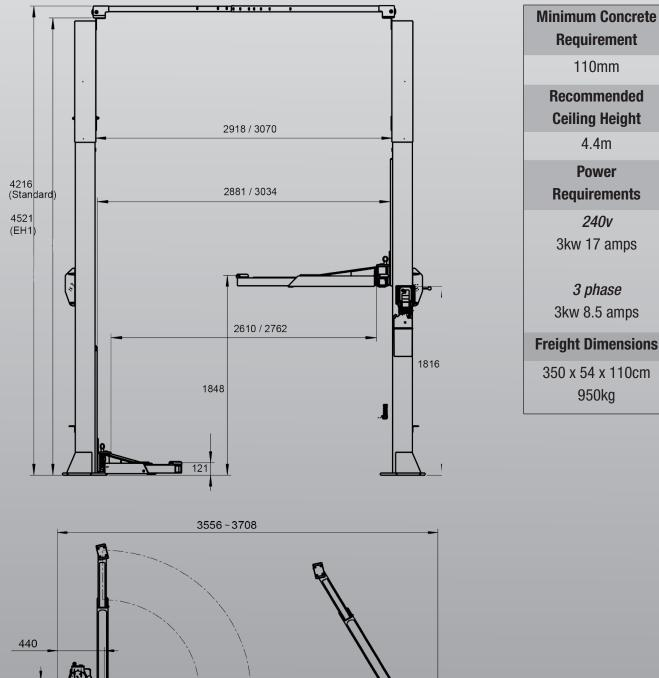
**Ceiling Height** 4.4m **Power Requirements** 240v 3kw 17 amps 3 phase 3kw 8.5 amps **Freight Dimensions** 350 x 54 x 110cm 950kg
