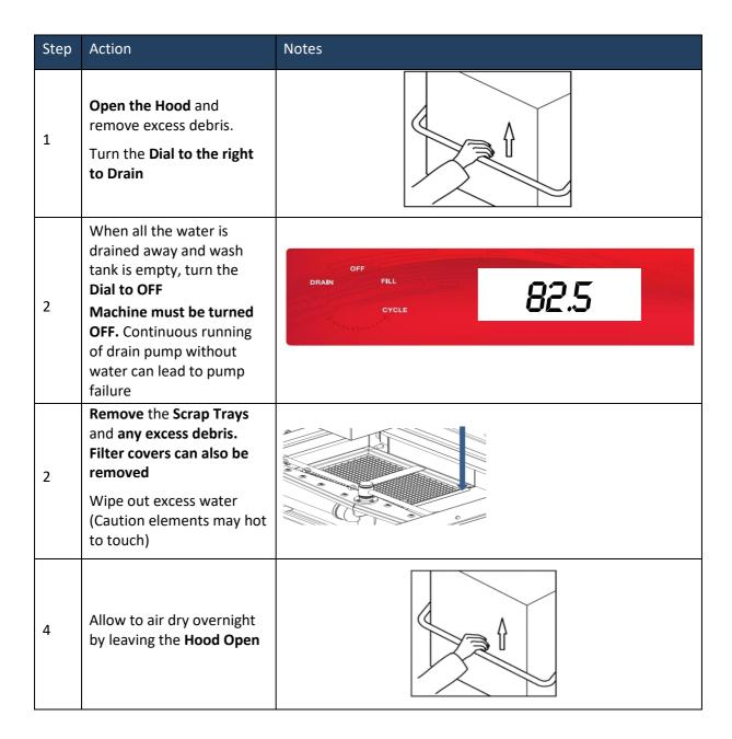
Note: Machine dial must be switched to OFF at end of day
