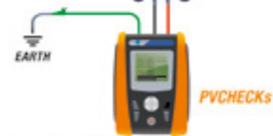
Insulation measurement with method "whole photovoltaic field"
