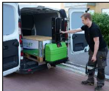
2. Pull the support legs out and lift the chassis up.
