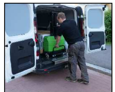
4. Push the InnoLift and the cargo into the van.
